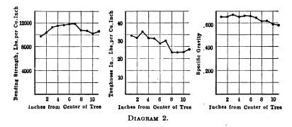
The three diagrams show the variation in the strength, toughness, and specific gravity (dry weight) of hickory at different distances from the center of the tree. In normal trees the strongest wood appears to be from 5 to 7 inches from the center and the toughest wood nearly at the center. Wood 3 to 7 inches from the center is generally high in mechanical properties.
